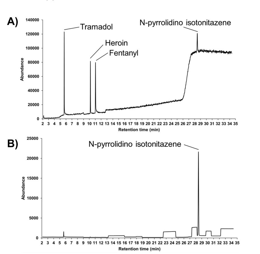
Figure 2. Exemplar results for Blind sample 20 for A) scan acquisition data and B) SIM acquisition data.
