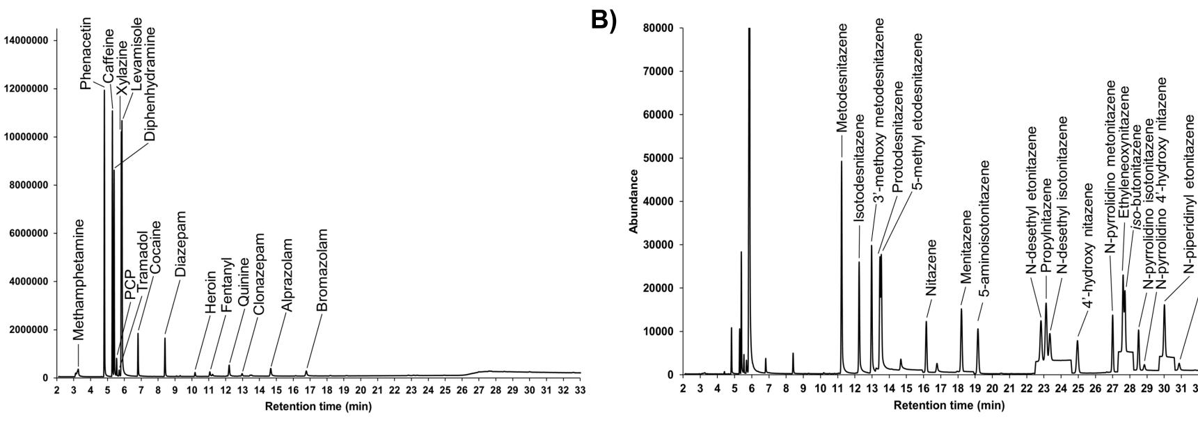
Figure 1. Comparison of A) scan acquisition data for the interferences and B) SIM acquisition data for targeted nitazene analogs.
